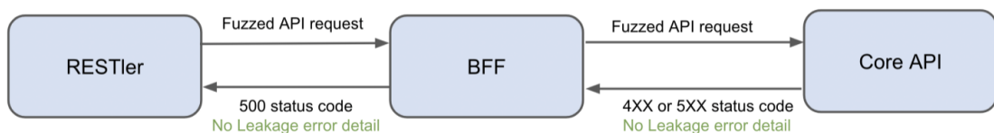
Figure 3.1: Good BFF and Good Core API
